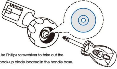
Use Phillips screwdriver to take out the back-up blade located in the handle base.
