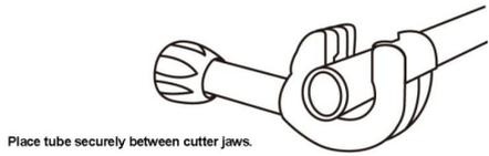
Place tube securely between cutter jaws.
