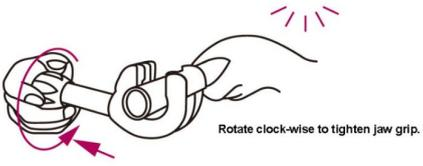
Rotate clock-wise to tighten jaw grip.
