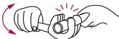
Tighten tool around the tube when needed.
